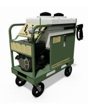
Incorporating an onboard electric-start diesel engine power supply with an hour meter, battery and charging system, there are no additional power requirements. With ample water and chemical (gas path) storage onboard, setup time is minimal. The TEWS system is designed to be pushed, driven or airlifted to the aircraft and placed into immediate operation.
