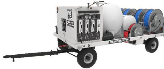
The system is designed to support large aircraft turbine engine compressor washing and all its components. Set up time is 15 minutes or less at the aircraft and a complete wash/rinse cycle duration of 25 minutes or less for all four engines.
