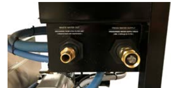
Plumbing connections for inlet water and sewer discharge made at rear of ECIN
