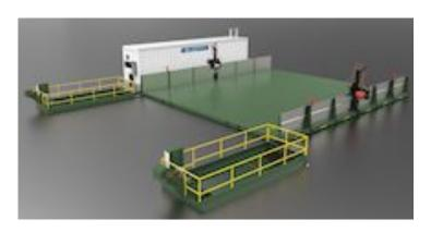
Hydropad wash rack; 40' wide X 45' long, drive thru design, Hydrosite equipment enclosure for wash and recycle equipment. Wash monitors, water cannons and Hydroblaster pressure washer with water and solids flowing to in-ground solids settling with drag conveyors for automatic solids removal. Example only....design
