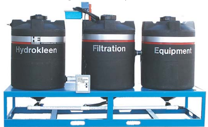
Filtration systems for recycling or pre-treatment for discharge to sanitary sewer
