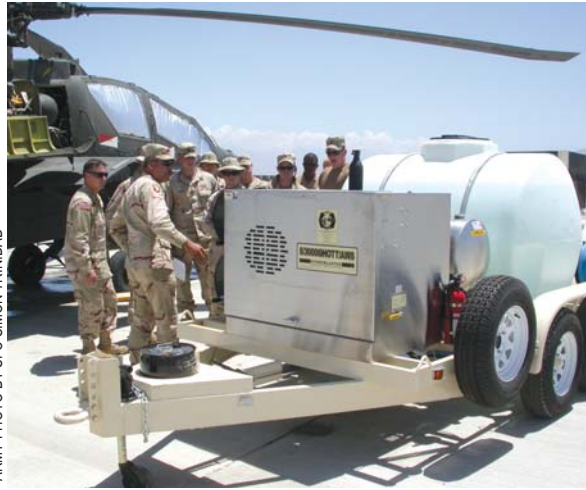
Troops receive new equipment fielding training on the "Hydroblaster" aircraft wash system (AWS) as part of their deployment.
