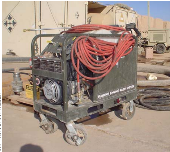
The turbine engine wash system or TEWS is a substitute for the antiquated Universal Wash System in the aviation unit maintenance formations.
