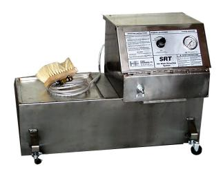
**Sump**: A 20 micron filter bag collects solids for disposal. Also a built in weir maintains solids in this compartment where system cleaning is centralized.
